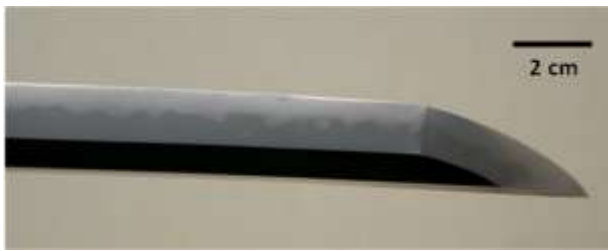
Figure 4. Top view of the sword (shown in fig.3) showing wavy pattern along the sharp edge.
